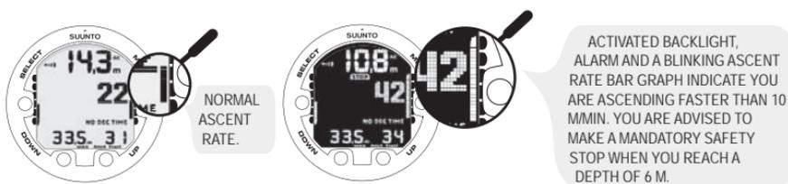
**WARNING** *DO NOT EXCEED THE MAXIMUM ASCENT RATE! Rapid ascents increase the risk of injury. You should always make the Mandatory and Recommended Safety Stops after you have exceeded the maximum recommended ascent rate. If this Mandatory Safety Stop is not completed, the decompression model will penalize your next dive(s). Continuous ascent rate violations will result in Mandatory Safety Stops. When Recommended Deep Stop is enabled, the length is indicated in seconds.*
