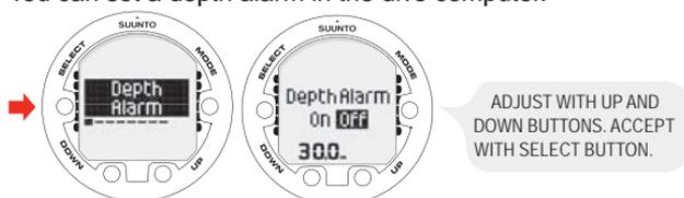
The depth alarm is factory-set to 30 m/100 ft, but you can adjust it according to your personal preference, or switch it off altogether. The depth range can be set from 3 m to 100 m/9 ft to 328 ft.
