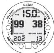
The change in your air consumption will be based on constant one second interval pressure measurements over 30 - 60 second periods. An increase in air consumption will influence the remaining air time rapidly, while a drop in air consumption will increase the air time slowly. In this way, an over optimistic air time estimation, caused by a temporary drop in air consumption, is avoided.
