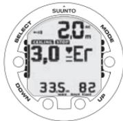
DECOMPRESSION DIVE, ABOVE CEILING. NOTE DOWNWARD POINTING ARROW, ER WARNING AND ALARM. YOU SHOULD IMMEDIATELY (WITHIN 3 MINUTES) DESCEND TO OR BELOW CEILING.
