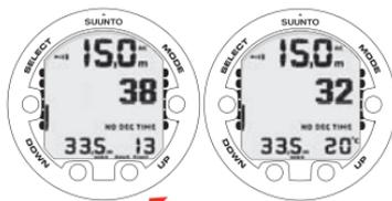
UP BUTTON TOGGLES BETWEEN DIVE TIME AND WATER TEMPERATURE.
