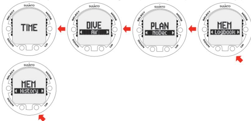
The dive time and date are registered in the Logbook memory. Always check before diving that the time and date are correctly set, especially after traveling between different time zones.
