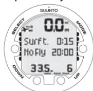
IT IS 15 MINUTES SINCE YOU SURFACED FROM A 6-MINUTE DIVE. THE PRESENT DEPTH IS 0.0 M. THE AIRPLANE SYMBOL AND NO-FLY VALUE INDICATE THAT YOU SHOULD NOT FLY FOR 20 HOURS.
